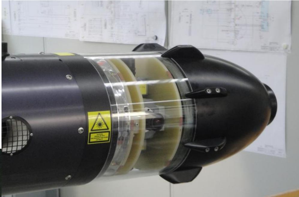
The inspection head, featuring 5 cameras and lighting
