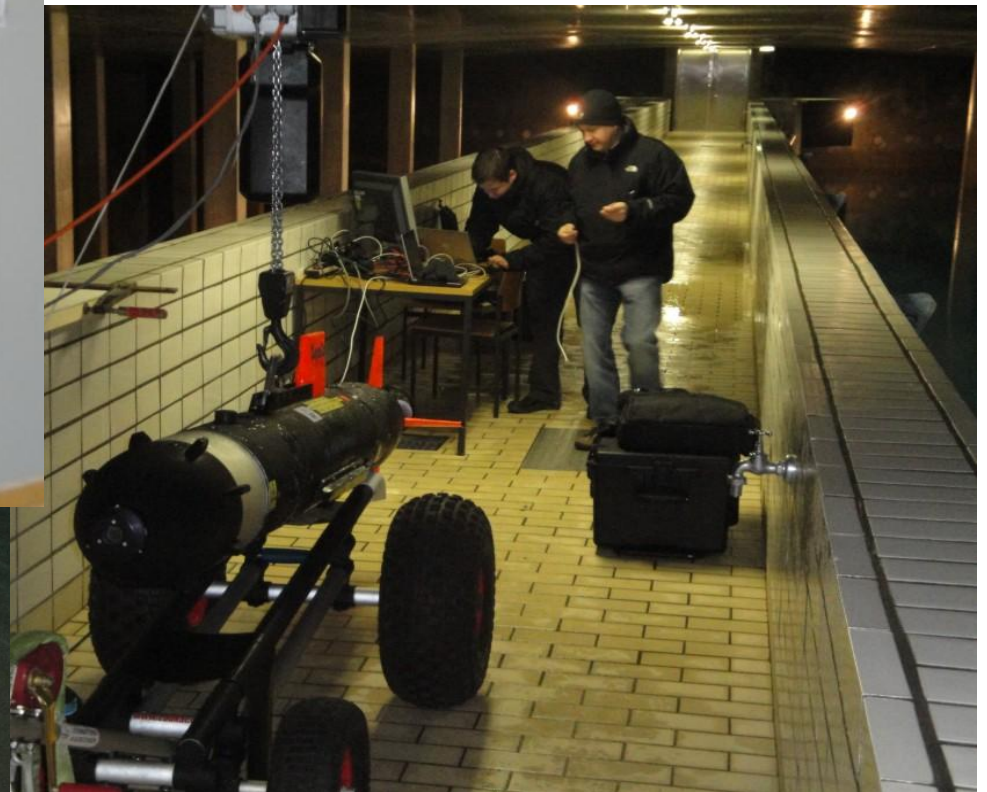
The inspection head, featuring 5 cameras and lighting
